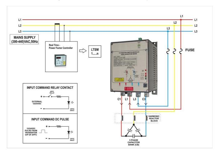
**Thyristor Switch Module (VTSM) for Capacitor Bank**
